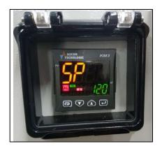
The instrument will automatically go back to its home screen after approximately 20 seconds. Ensure the lid is clipped shut to avoid any damage to control unit.
